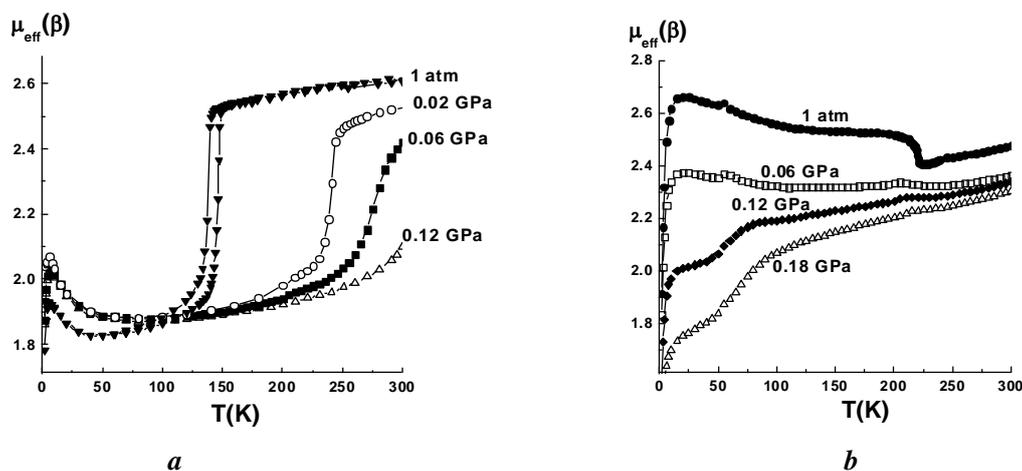
**Fig. 1.**  $\mu_{\text{eff}}$  versus  $T$  plots at different pressures of  $\text{Cu}(\text{hfac})_2\text{NN-Pz}^{\text{Me}}$  (a) and  $\text{Cu}(\text{hfac})_2\text{NN-Pz}^{\text{Et}}$  (b).
